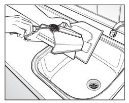
Clean the fabric conditioner channel with a brush and hot water. Liquid starch can cause the siphon to become clogged. Make sure that you clean the siphon and siphon tube particularly thoroughly after using liquid starch a few times.
